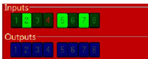
In keypad mode (K) move the X-axis into the proximity target using the left arrow on the keypad. The proximity switch will have a red LED lit until it comes across the proximity target, when it will turn off. Moving off the top of the target should cause the LED to come back on. This should also be evident in the ShopBot position screen when looking at input “2”, the light will turn from black (normally closed) to green (open).
