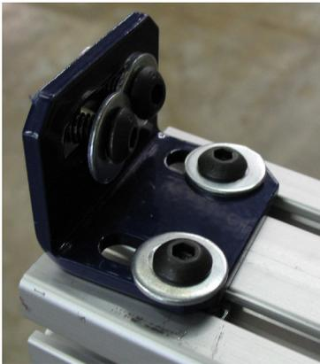
Pre-assemble tool bar mounting bracket with four 5/16x3/4" button head screws, 5/16" flat washers, and 5/16" T-nuts.
