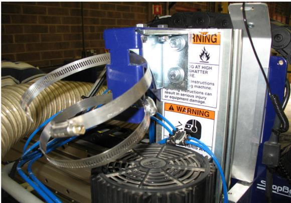
Pry black plastic cap from top of Z-axis with a flat head screwdriver. Pre-assemble two 1/4-20x1/2" button head screws and two 1/4-20 T-nuts through the dust hose guide bracket. It may be necessary to slit the top sticker down the left side of the Z-axis extrusion. Slide the bracket down into the extrusion and tighten the bolts. Replace black plastic cap.
