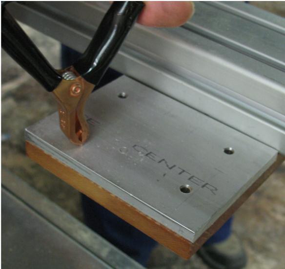
Touch the grounding clip to the fixed Z zero plate. Input "1" should light up green each time that the grounding clip contacts the fixed Z zero plate.
