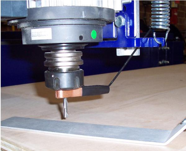
When the bit is located over the area needed to set as zero, type "C2" ("Zero Z-Axis w/ Z zero Plate").
