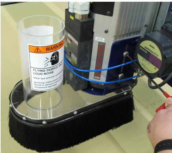
Securely tighten dust skirt to the side of the spindle with four M6x10mm socket head screws.
