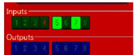
Release the button. The drawbar will close (captures tool holders). With the tool holder in place, input "7" will be lit and input "8" will go off.
