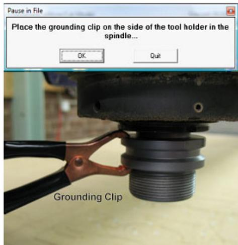
Place the black grounding clip on the tool holder in the spindle.
