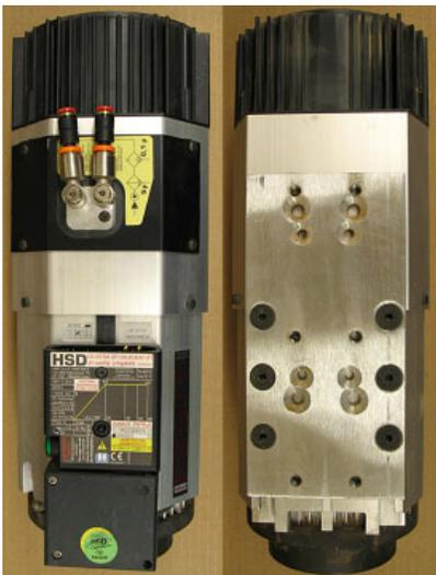
The ShopBot ATC is equipped with a 5HP HSD spindle. The spindle is cooled by an electric fan, but also has air-cooled lower bearings. The air required for cooling the lower bearings is 60 psi (4 bar).
