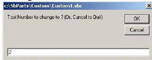
Insert bit into conical tool holder and place it in the desired tool holder location. Type C1 to run the custom number 1 "Change Tools" routine. A screen will ask which tool should be selected. Once that tool is entered, click "OK" and the ATC will drop off the current tool being held and select the desired tool.
