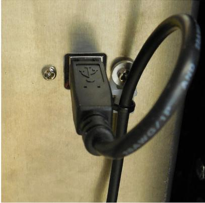
Plug in the provided USB cable into the control box connector, and make a loop in the cord for strain relief. Fasten the cord to the zip tie mount. Plug in the USB cable to the computer only after the software is installed on the computer.
