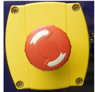
Note: Input #4 will flash red on the computer screen and the ShopBot control software will not allow the ShopBot to move if the emergency stop is not connected.
