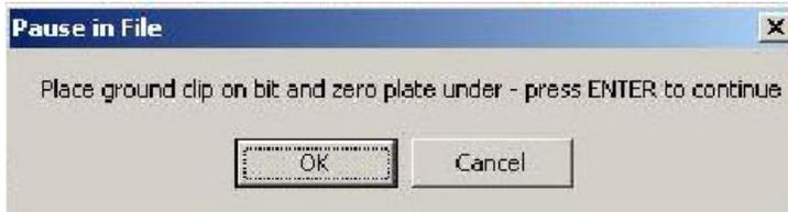
Place the Z zero plate under the bit and place the grounding clip on it. Click "OK" when both are in place. The Z-axis will touch off the plate twice, and record this distance for use on all the tools until this Z offset is reset.
