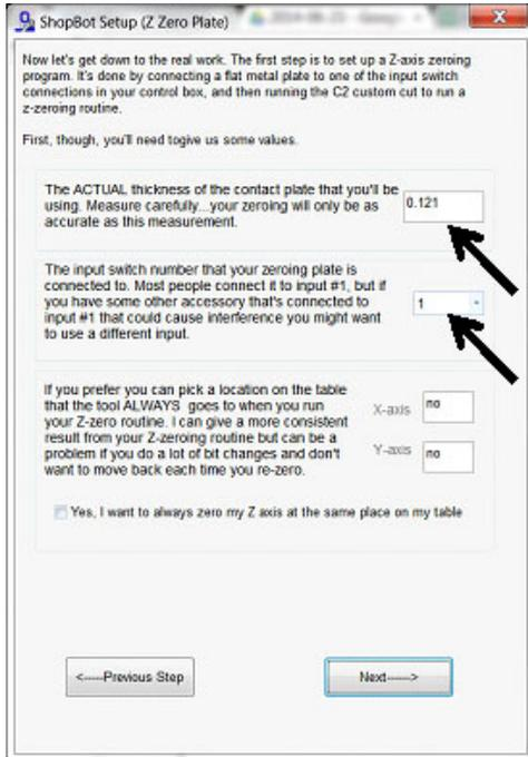
In the “ShopBot Setup (Z Zero Plate)” screen, measure the thickness of the plate and enter that value. Make sure the input switch is set to “1”. DO NOT check the “Yes, I want to always zero my Z axis at the same place on my table”. Click “Next”.
