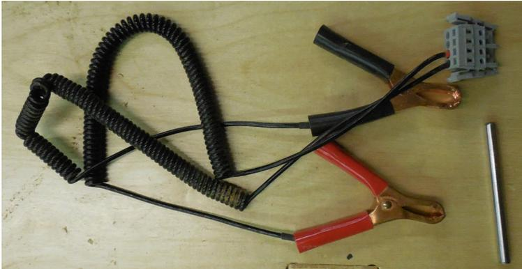
Obtain the calibration clip and drill rod that came with the ATC. Connect the Wago plug to the mating plug on the Z-axis. The grounding clip is also attached to this same plug.
