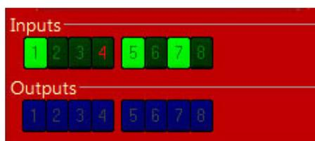
Connect the Z zero plate and the calibration clip. Input "1" should light up green on ShopBot position screen as shown.
