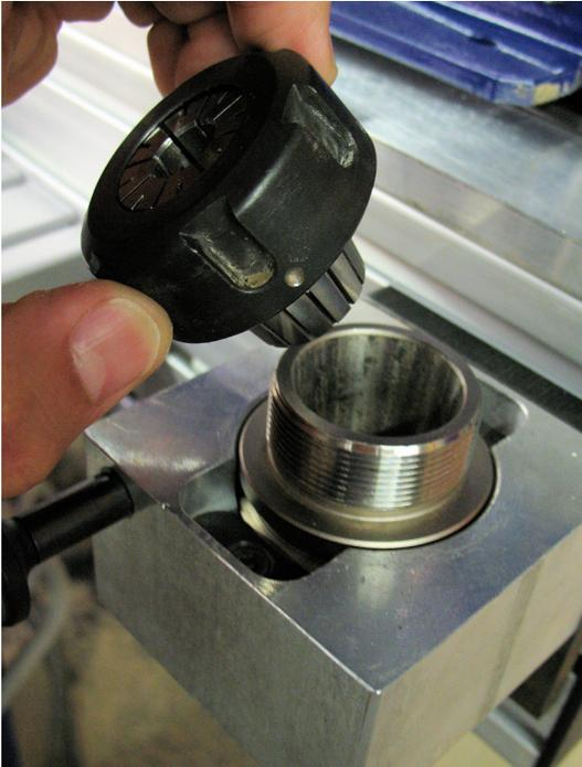
Snap the collet into the collet nut and thread the assembly onto the tool holder. Ensure the collet is the correct size for the bit needed.
