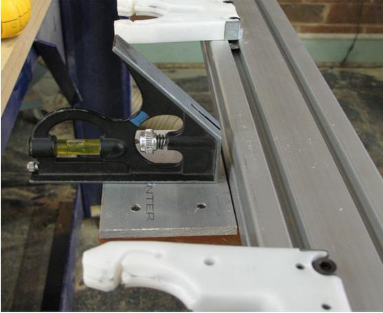
Level the tool bar by placing a level on the fixed Z zero plate (pre-attached to tool bar), then securely tighten all 5/16" button heads in tool bar mounting bracket.
