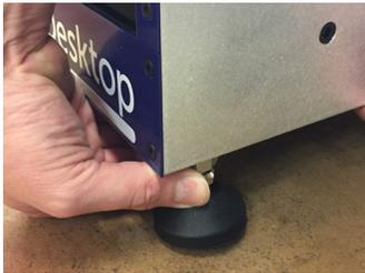
Use the levelling feet to level the tool on the workbench surface.
