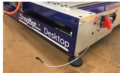
Make sure all cables and dust collection have been disconnected from the tool.
