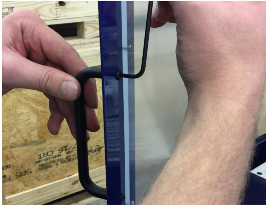
Attach the Top Support (the one with the magnets) to the front of the enclosure using 8 BHSCS M6-1.0x10mm, 4 on each side. Do not tighten the bolts at this time.
