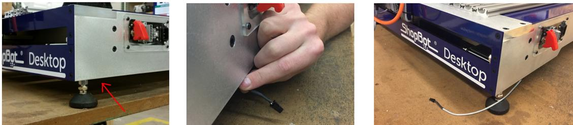
Locate the interlock connector at the rear of the tool. It will be under the tool near the red power switch. Leave it attached, but extend it and route it around the back foot, so that it is laying to the side of the tool for accessibility during assembly.
