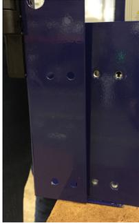
The door assembly flange should be in front of the front bottom support.
