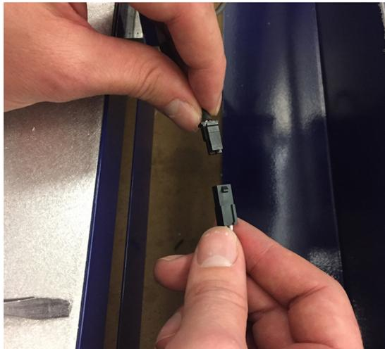
To confirm proper connection and operation of your enclosure, connect to the ShopBot Desktop MAX with the sb3 software. When either door is open, you will see a yellow indicator that says “DOOR!” in the DRO display.
