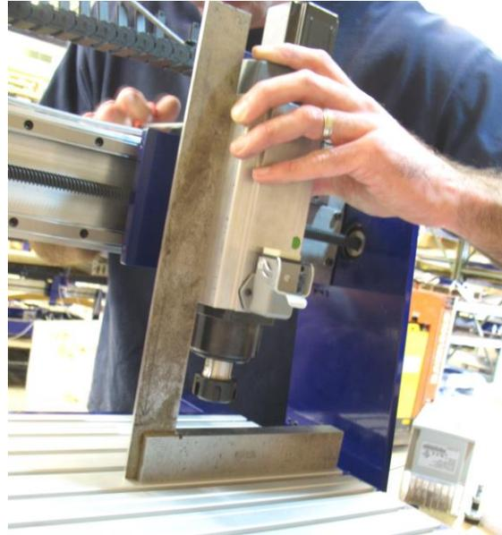
Checking the spindle for square
